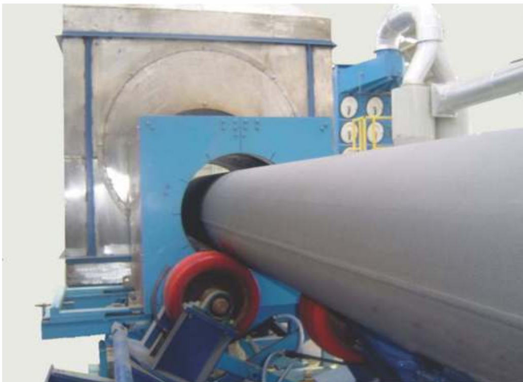
Schematic of Induction Heating for Pipe Coating
