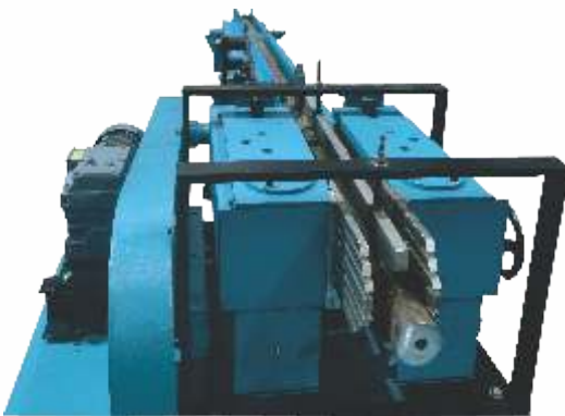
Infeed Chain Conveyor with Tractor Drive
